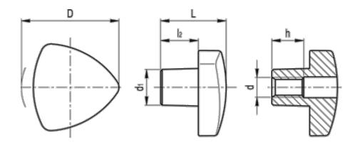
$\begin{array}{lll} D & = 40 \\ d & = M8 \\ d1 & = 14 \\ h & = 13 \\ L & = 26 \\ l2 & = 14 \\ Weight (g) = 90 \end{array}$
